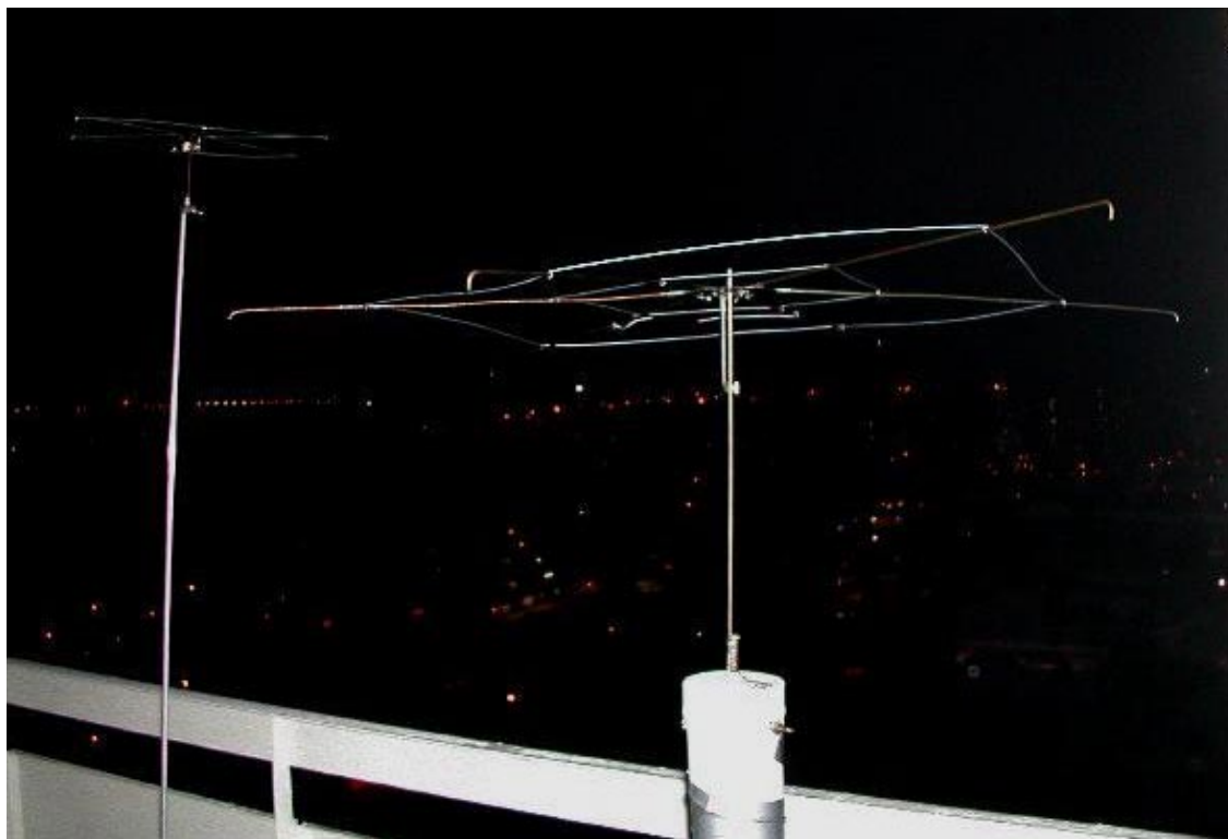
The antennas for 10 m and 20m band on a balcony in 19 th floor of apartment building in Etobicoke.
