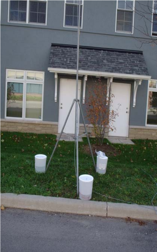
The buckets are filled up with water and sit on bolts that are attached to the tripod. When not in use the pails double as general storage for our equipment.
